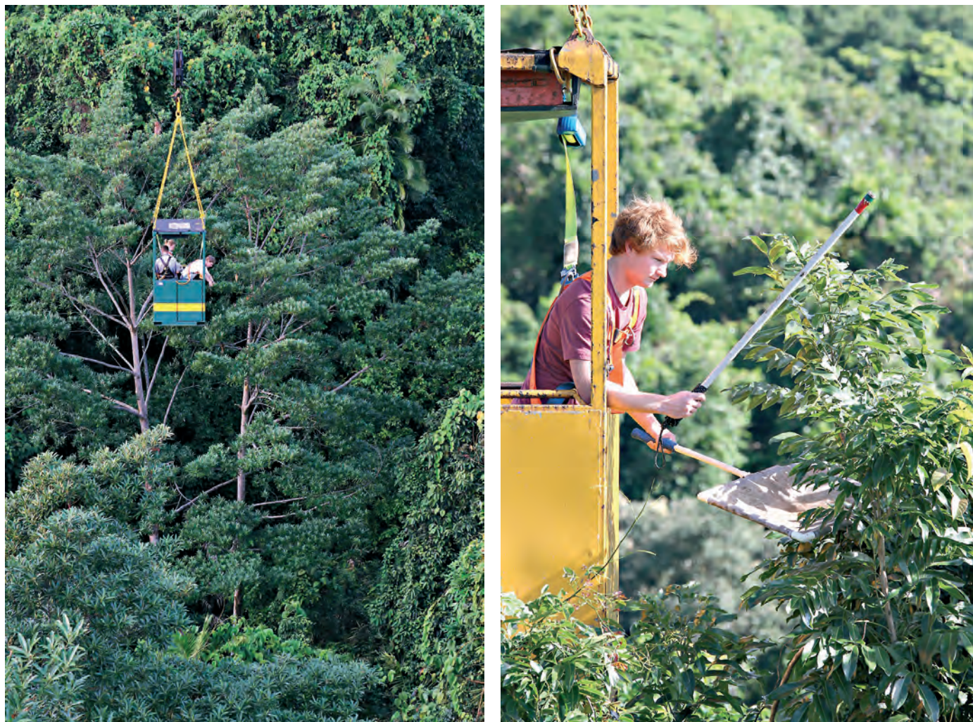
FIG. 3. The 47 m tall Australian Canopy Crane at the Daintree Rainforest Observatory provides scientists with canopy access across a 1-ha area of lowland rainforest (photos by P Byrnes)
